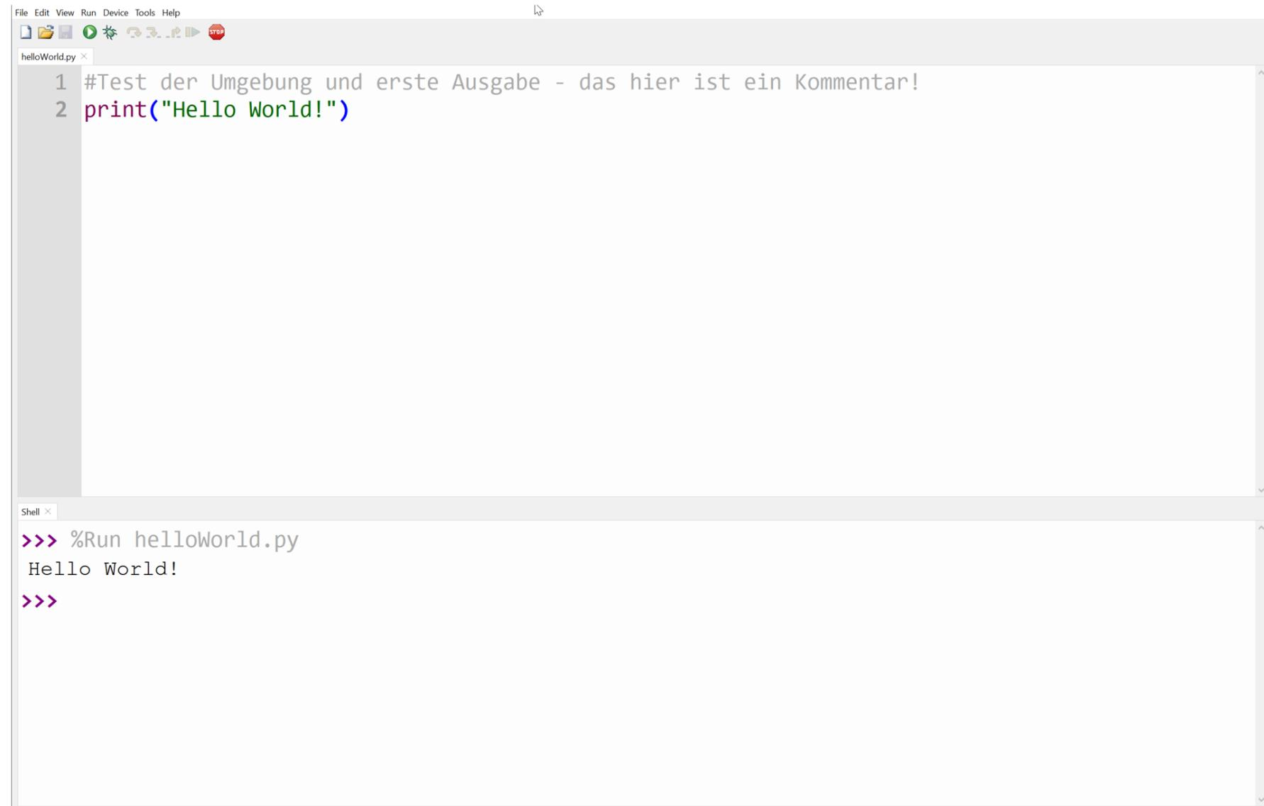
The screenshot displays the Thonny IDE interface. At the top, there is a menu bar with 'File', 'Edit', 'View', 'Run', 'Device', 'Tools', and 'Help'. Below the menu bar is a toolbar with icons for file operations, running, and stopping. The main editor window shows a Python file named 'helloWorld.py' with the following code:
