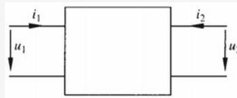
$$\begin{aligned} u_1 &= h_{11} \cdot i_1 + h_{12} \cdot u_2 & u_{BE} &= h_{11} \cdot i_B + h_{12} \cdot u_{CE} \\ i_2 &= h_{21} \cdot i_1 + h_{22} \cdot u_2 & i_C &= h_{21} \cdot i_B + h_{22} \cdot u_{CE} \end{aligned}$$
