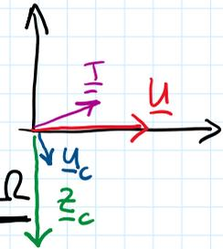
$\underline{U}_C = \frac{\underline{Z}_C}{\underline{Z}_C + \underline{Z}_R} \cdot \underline{U} = \frac{-j 1693,14}{-j 1693,14 + 10k\Omega} \cdot 10V =$
